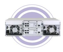
EonPath multipathing drivers are now available for application servers running Windows, Solaris, or Linux operating systems. EonPath provides multipath IO function by recognizing and managing the fault-tolerant data paths to an individual RAID volume. Greater reliability is achieved through the path failover mechanism in the event of cabling component failure. The EonPath also comes with load-balancing algorithms which help accelerate the throughput across host-storage data links.
